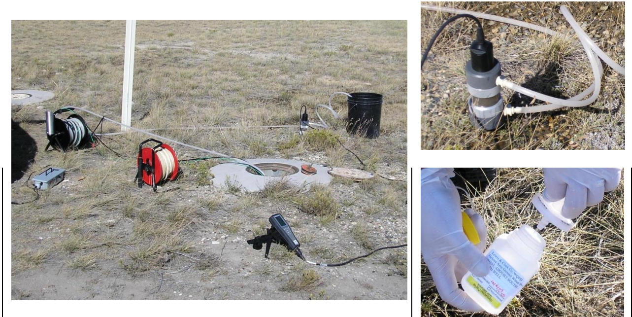
Figure 4-2 Monitoring Well Sample Collection
