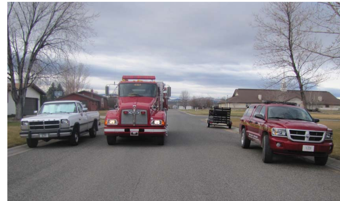
CH 5 FIGURE 4B— High density neighborhoods built in the City must have adequate road widths to provide for on-street parking while keeping roads passable for evacuation and emergency vehicle access.
