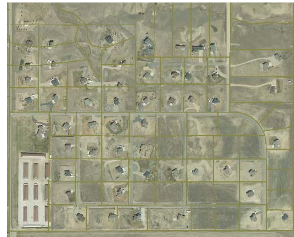
CH 2 FIGURE 6— Emerald Ridge Subdivision where development of 50 homes on 1-acre lots has dropped the water table up to 10 feet per year due to lack of aquifer recharge.
